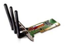
With MIMO technology, WML-8315 enables you to connect to wireless networks at farther distances than before. WML-8315 has two antennas for signal reception and one antenna for high power signal transmission. Not only the connection distance is enhanced, but also the "dead spots" in the network will be reduced. For WLAN security issues, WML-8315 supports 64/128-Bit WEP / WPA and WPA2 data encryption that protect your wireless network from eavesdropping.
